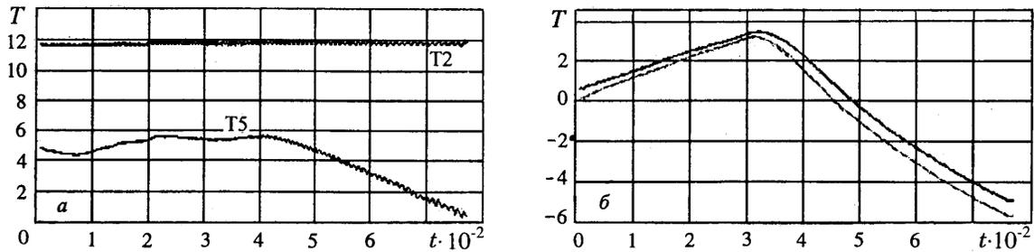
Fig. 5. Investigation of the influence of heat-removal conditions (T7 and T8) on the temperature of the evaporation zone (T2) of the heat pipe with a heat hydraulic accumulator.  $T$ ,  $^{\circ}\text{C}$ ;  $t$ , sec.
