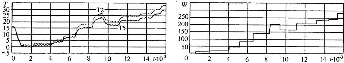
Fig. 2. Tests of the heat pipe without regulating elements: temperatures of the evaporation zone (T2) and the condensation zone (T5) and power supplied to the evaporation zone vs. time.  $T$ , °C;  $W$ , W;  $t$ , sec.
