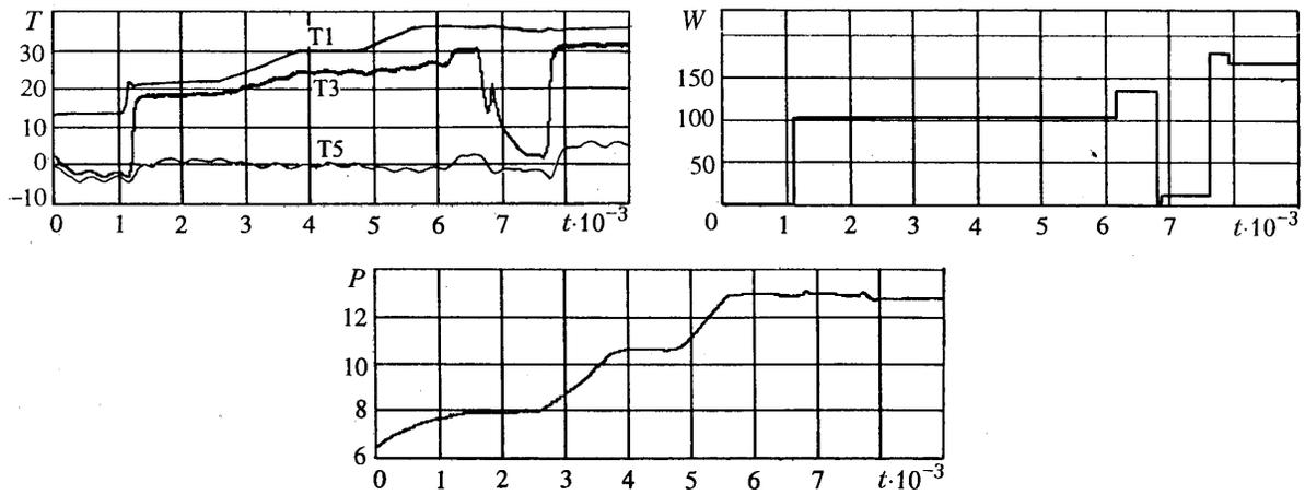
Fig. 4. Investigation of the possibility of specifying the temperature of the evaporation zone of the heat pipe with a heat hydraulic accumulator (T1) by changing the pressure in the heat hydraulic accumulator.  $T$ , °C;  $W$ , W;  $P$ , bar;  $t$ , sec.
