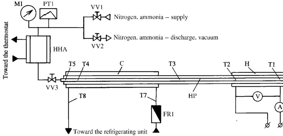
Fig. 1. Pneumatic hydraulic circuit of the experimental setup.
