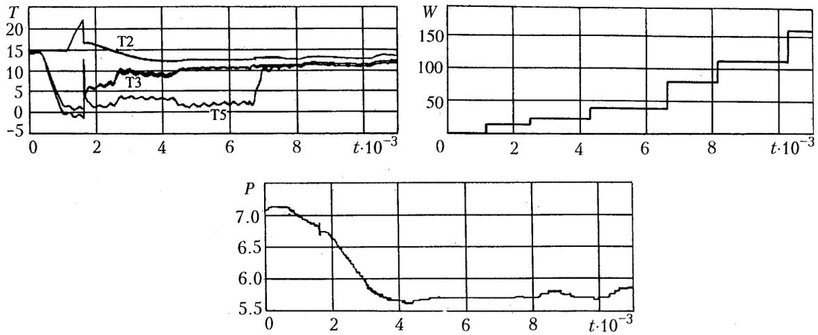
Fig. 3. Regulation of the temperature of the evaporation zone of the heat pipe (T2) using the heat hydraulic accumulator for a variable heat flux in the evaporation zone in the course of the experiment.  $T$ , °C;  $W$ , W;  $P$ , bar;  $t$ , sec.
